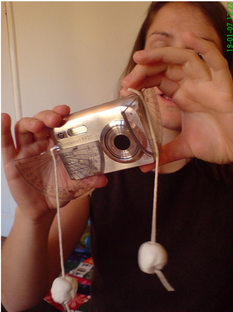
Figure 10. The 7D Tiltometer – Protractors and Plumb Bobs.
